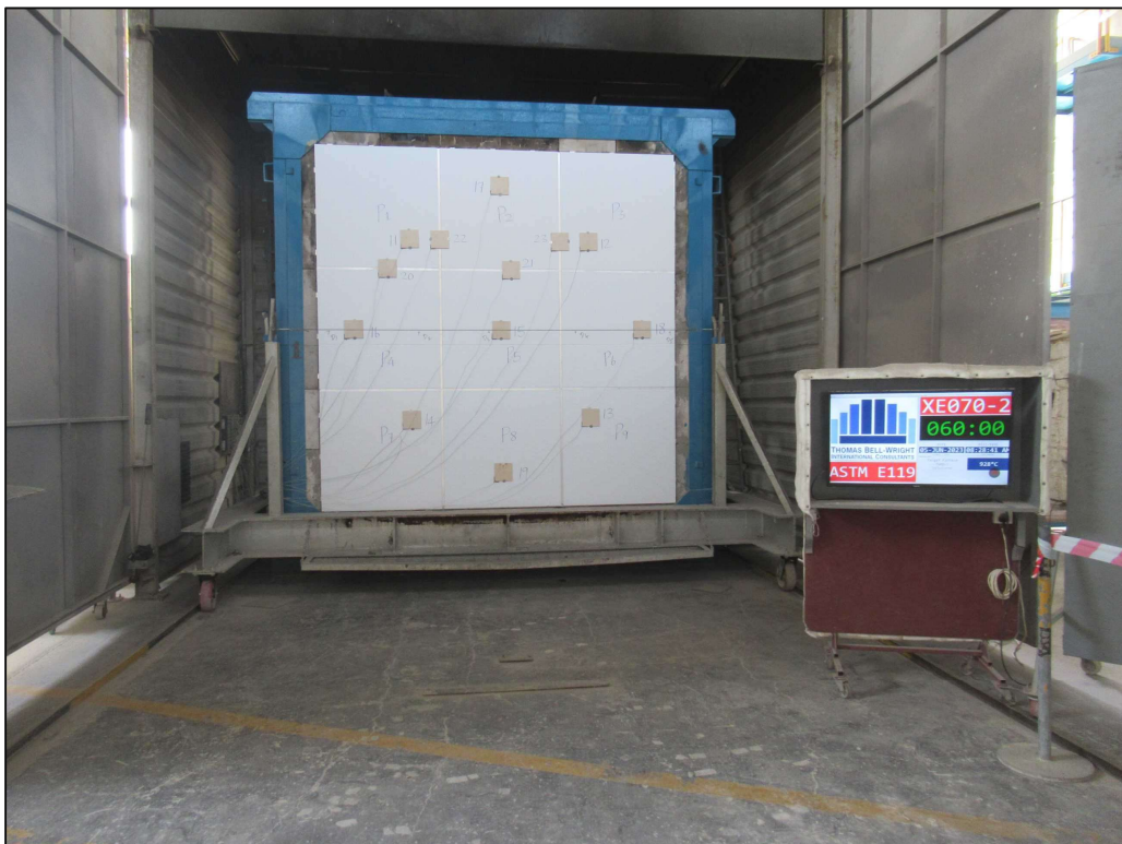
Picture 10: The unexposed face of the specimen after 60:00 minutes.
