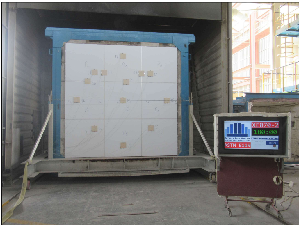
Picture 12: The unexposed face of the specimen after 180:00 minutes.
