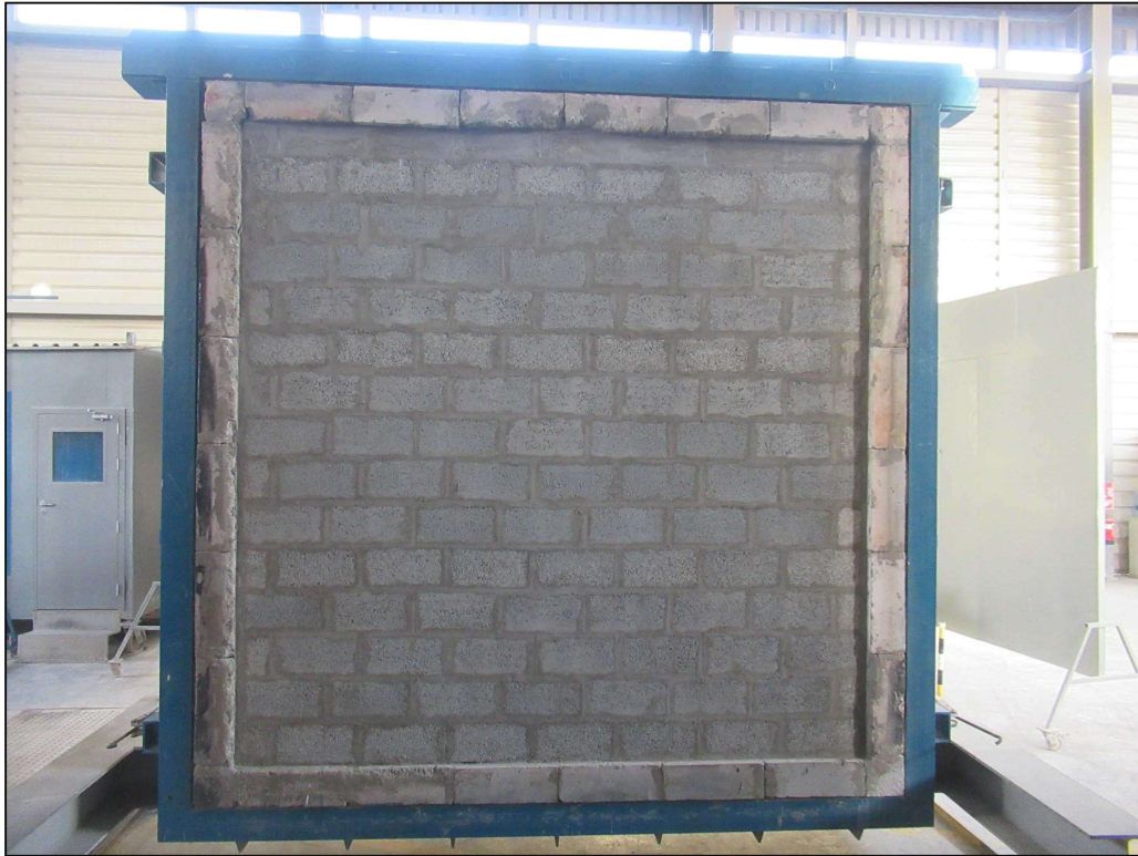
Picture 7: The exposed face of the specimen prior to the start of the test.
