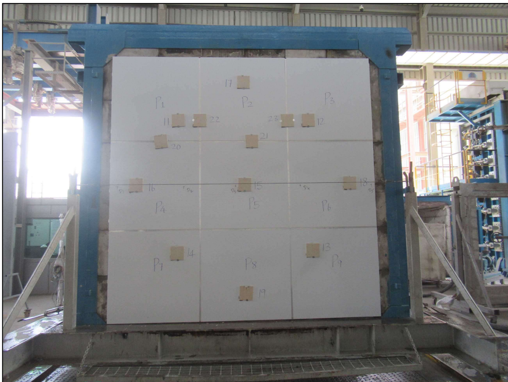
Picture 16: The unexposed face of the specimen after the hose stream test.
