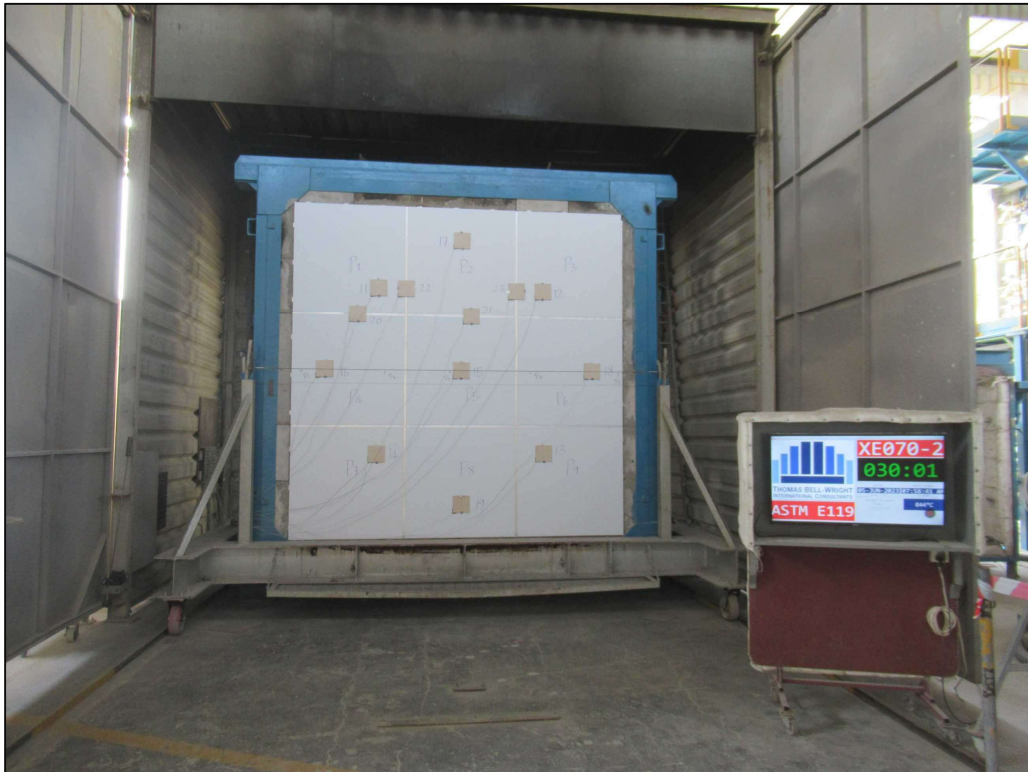
Picture 9: The unexposed face of the specimen after 30:00 minutes.
