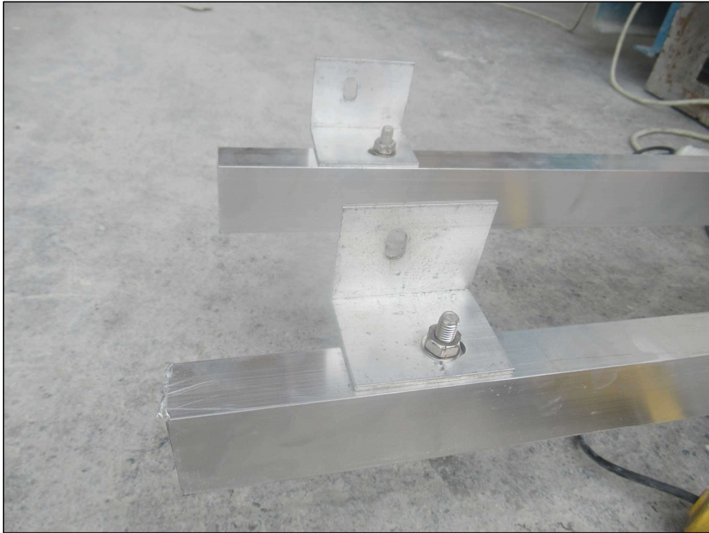
Picture 1: The brackets fastened to the runners.
