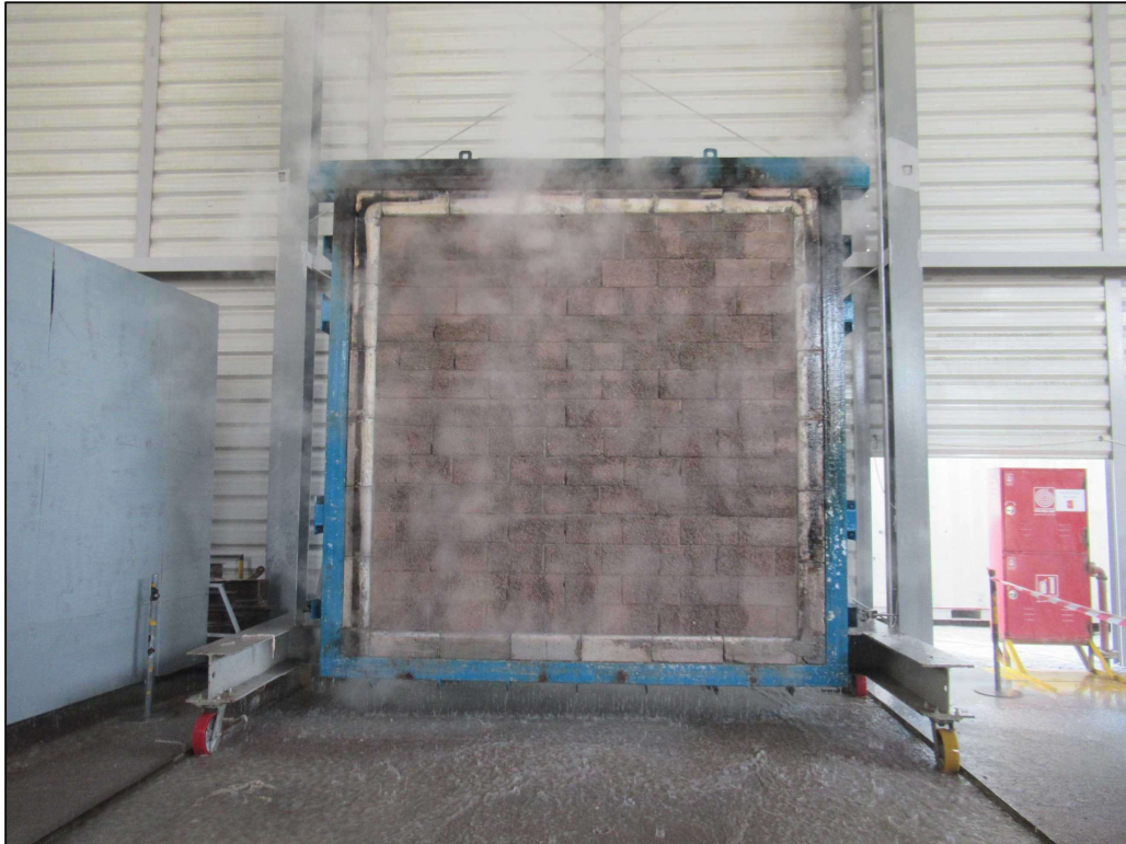
Picture 15: The exposed face of the specimen after the end of the hose stream test.
