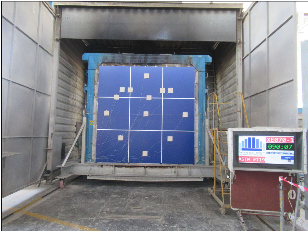
Picture 11: The unexposed face of the specimen after 90:00 minutes.
