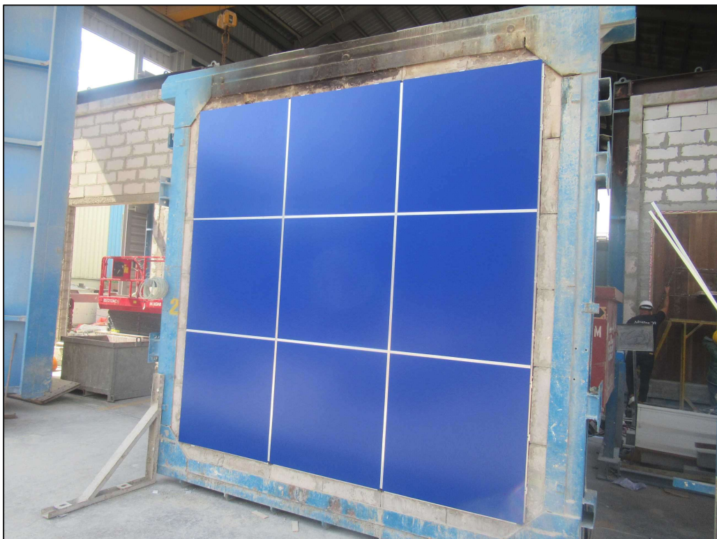
Picture 6: The specimen after the U-channels were fastened to the runners at the panel gaps.
