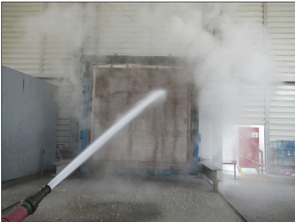
Picture 14: The exposed face of the specimen during the hose stream test.
