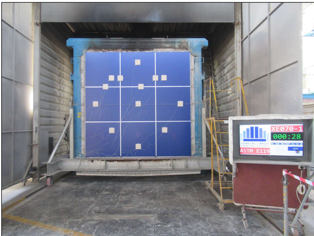
Picture 8: The unexposed face of the specimen after the start of the test.
