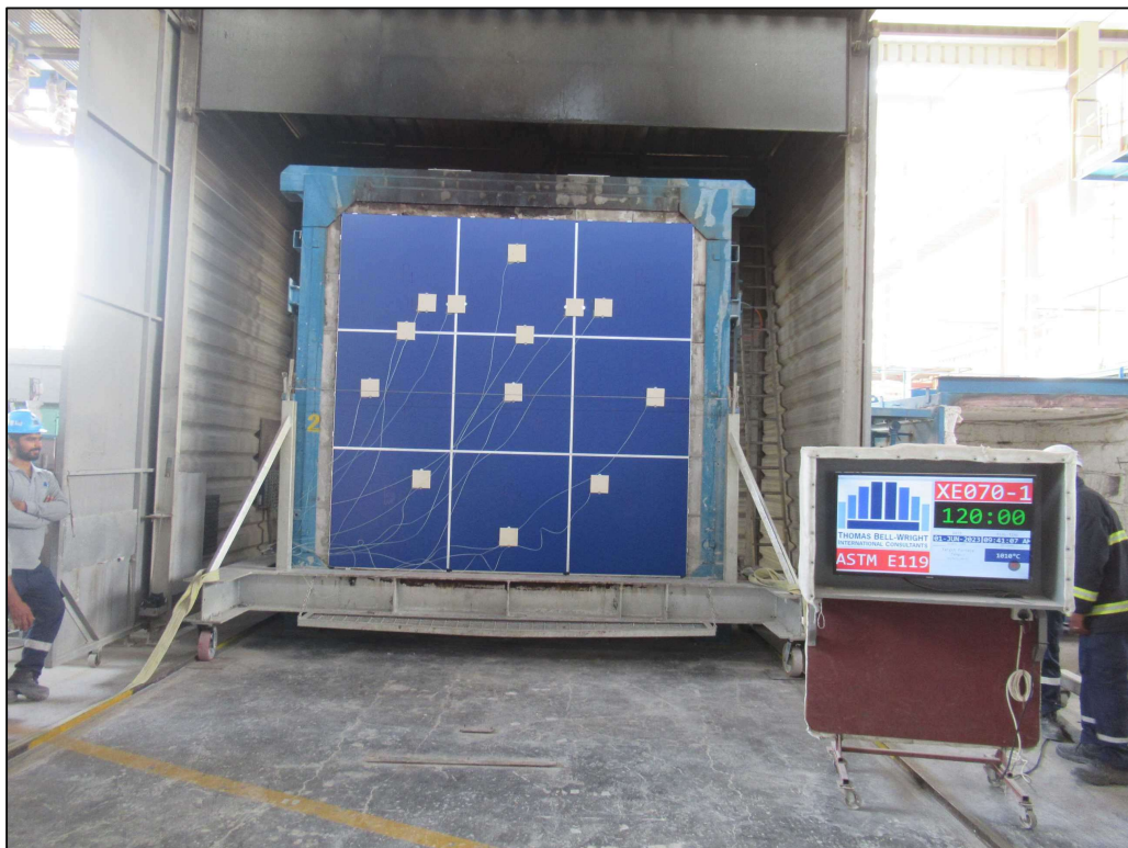
Picture 12: The unexposed face of the specimen after the end of the fire endurance test at 120:00 minutes.
